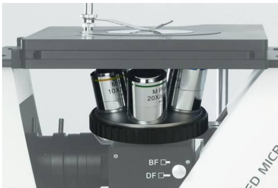
Dark field objective, Make observation in dark & bright field.
